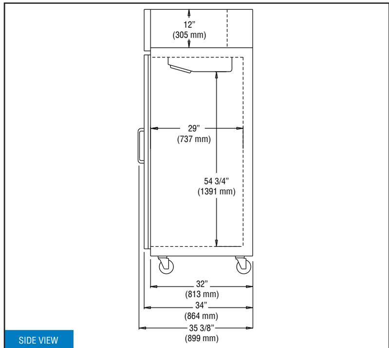
**IMPORTANT NOTE:** If the cabinet is located directly against a wall and/or under a low ceiling, a minimum clearance of 12" is required.
